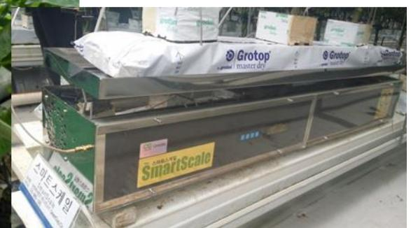
Precise irrigation control by load cel)
